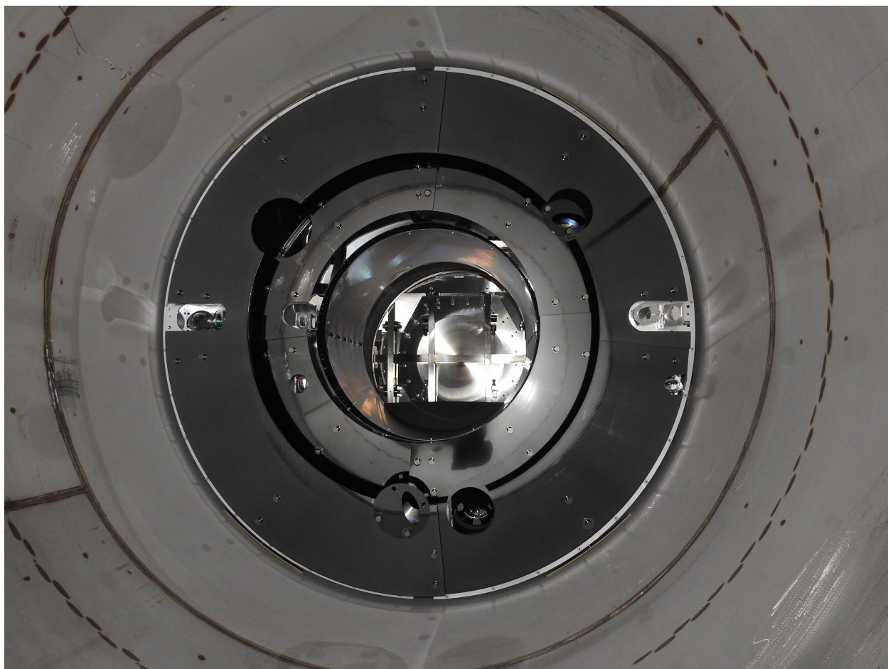
Figure 4.7. Photo showing the completed installation of the additional PCal periscope panels which provide full coverage. The Oplev nozzle baffles are also visible just to the left and to the right of the 6 o'clock position.
