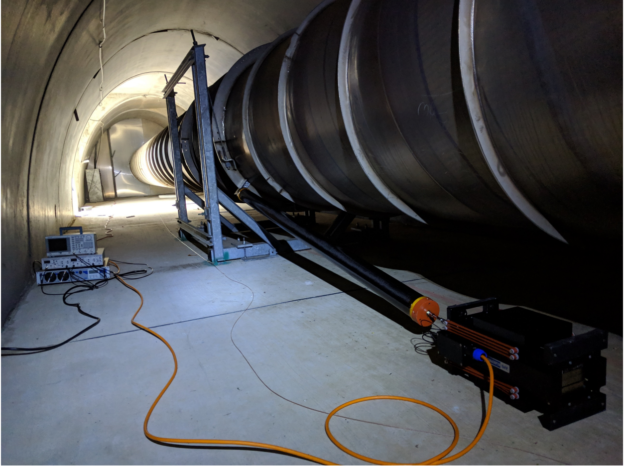
Figure 6.4. APS 113 Electro-Seis shaker with carbon fiber connecting tube used to perform driven measurements of the beamtube.
