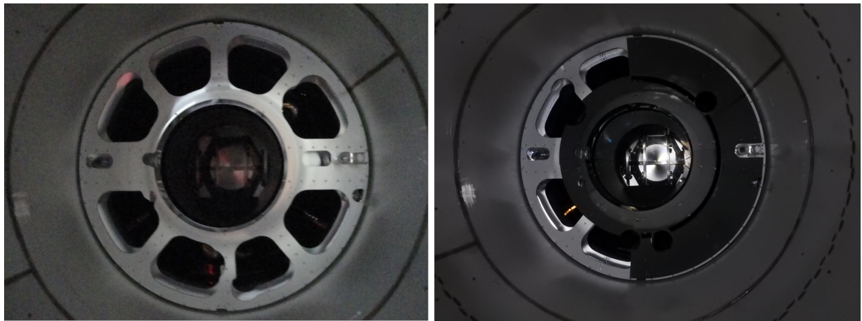
Figure 4.6. Photo showing the PCal periscope before (left) and after (right) installing SLiC baffles.
