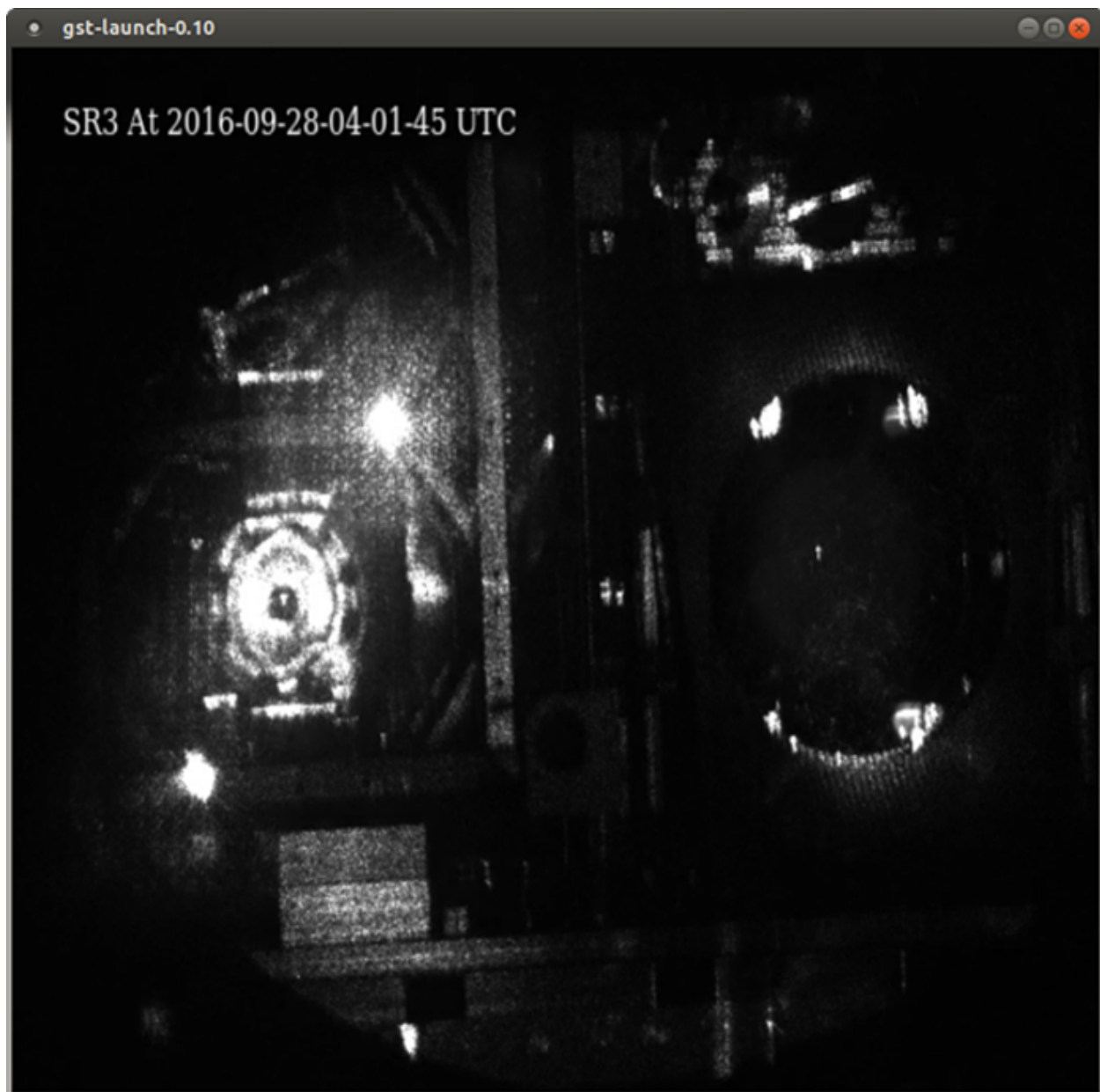
Figure 4.1. Photo taken in full lock of optics in HAM5. Glints can be seen on the suspension structure, ballast masses on the table, and earthquake stops.
